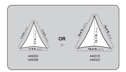
Identify attachment points that can withstand occasional windy conditions. Possible points of attachment may include reinforced fascias, trees or secured posts.
